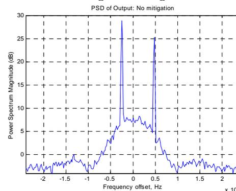
Figure 3 – 25 kHz DAMA SATCOM SOI corrupted by two CW interferers. The Signal to Interference power Ratio (SIR) is -10 dB, and the Signal to Noise power Ratio (SNR) is 2 dB. Pre-FEC BER =  $5 \times 10^{-1}$ .
