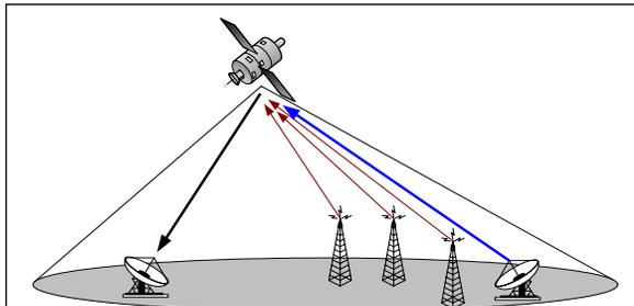
Figure 3 – Narrowband interference (incidental or intentional) often corrupts DAMA SATCOM signals because of the satellites' wide beams. Terrestrial emitters' signals couple into the satellite uplink and are downlinked along with the signals of interest.
